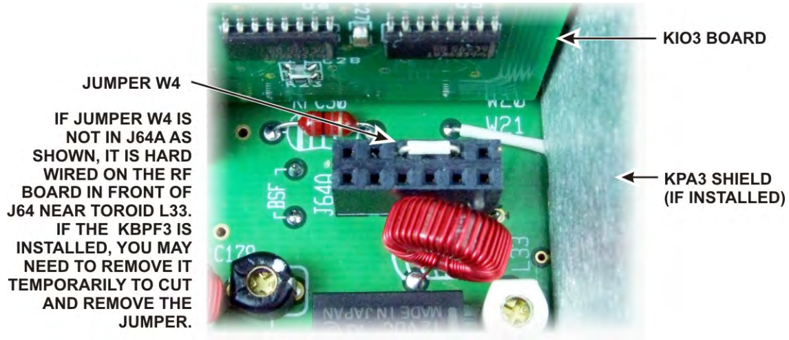
Figure 45. Jumper W4 on the K3 RF Board.
